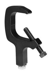
The Mega-Clamp is the world's new standard theatrical lighting C-Clamp. The Mega-Clamp is created from high tensile, aircraft grade, extruded aluminum; so it's both stronger and lighter than cast iron damps. The Mega-Clamp's safety factor far exceeds industry standards, breaking at over 2-1/2 tons at an independent testing laboratory. It is half the weight and twice as strong as most cast iron damps.
