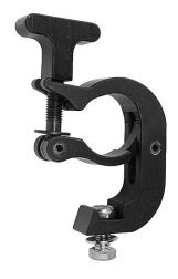
The TC Clamp will fasten from 2" OD to 1.5" OD tube. The TC Clamp has a 2-1/2" T-handle so no tools are required to fasten to the pipe.  $1.25'' \times 1/2"-13$  TPI Grade 8 fastener, Nylock Nut and 1" diameter Belleville Spring washer are provided for connecting your load. Dimensions: 4-5/8" Tx 4"W x 1-3/16" thick. Safe Vertical Working Load 450 Pounds, (200 KG). Weight is 1.22 pounds (.55 KG)
